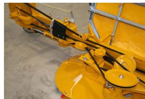
4. Now follow the belt through from the **bottom** of the Ø260 Drive pulley up and around the small Vee Idler, and back to the **RH / Front** of the Ø390 Driven pulley.
